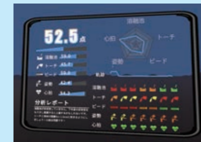
▶ In addition to measuring the stability of the weld pool, the system also analyzes and evaluates the movement of the welding torch and the posture of the welder
